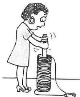
Fig. 4.50, It is more difficult to push the magnet into a coil with many loops because the magnetic field of each current loop resists the motion of the magnet.
