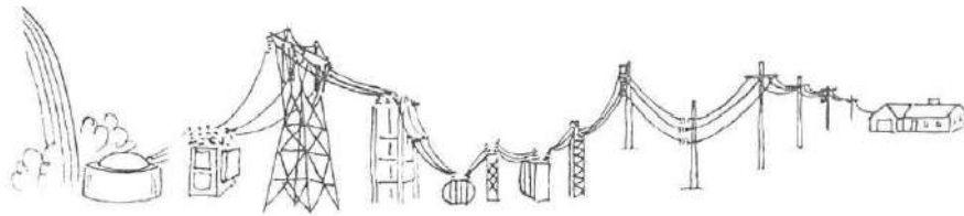
Fig. 7.18 Voltage generated in power stations is stepped up with transformers prior to being transferred across country by overhead cables. Then other transformers reduce the voltage before supplying it to homes, offices, and factories.
